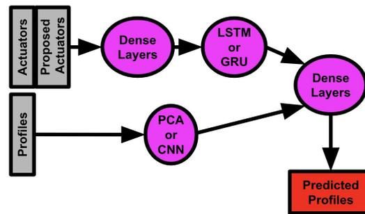
Model architecture: Principal Component Analysis or a Convolutional Neural Net extracts info from profiles, while a Recurrent Neural Net processes actuators.
