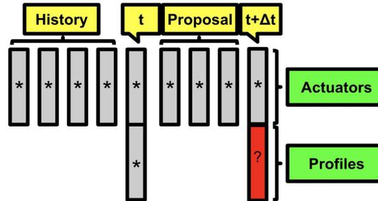
Format for the input to the model. Actuators (top) are specified by the operator and therefore are considered known at all timesteps. Profiles (bottom) are predicted by the algorithm 180 ms into the future.
