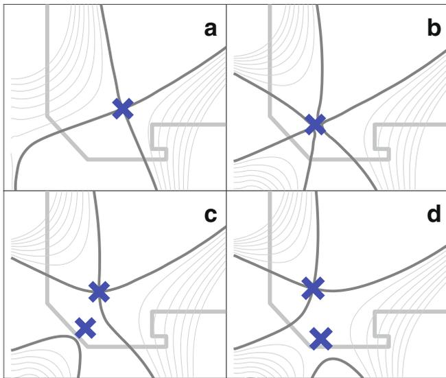
Fig. 1. (a) DIII-D standard x-point divertor configuration. (b) Perfect snowflake with a single, second-order null. (c) The snowflake-plus configuration with secondary x-point in the private flux region. (d) The snowflake-minus configuration with secondary x-point in the low-field-side scrape-off-layer.
