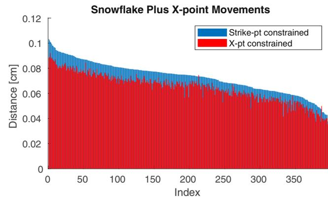
Fig. 4. Total distance moved by the x-points in the snowflake plus configuration when constraining the strike point positions only, versus constraining the x-points via Eq. 8.
