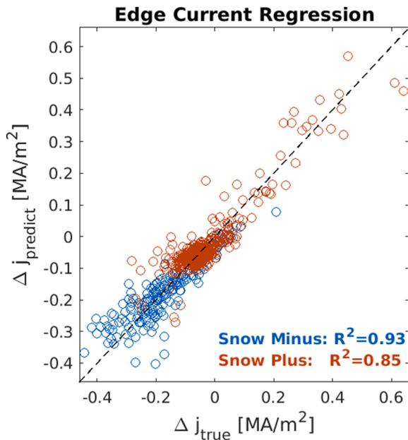
Fig. 6. Linear regression estimates for the change in the equilibrium edge current using the movement of x-points as predictor variables.
