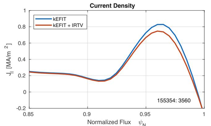
Fig. 5. Change in the parallel edge current density as the IRTV constraint is applied.
