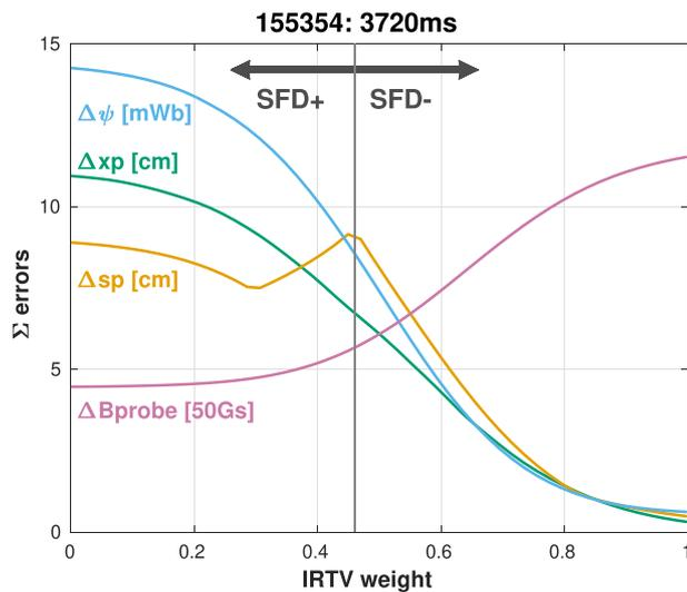
Fig. 7. Equilibrium fitting tradeoff for DIII-D 155354, the same example as shown in Fig. 2b, between the magnetic probe errors and the IRTV-inferred characteristics: strike point positions, flux of the secondary x-point, and x-point positions.
